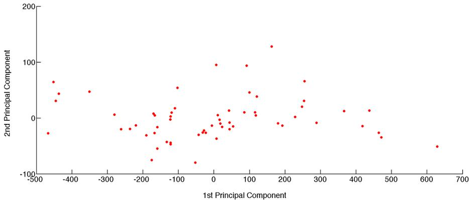
Figure 14: Distribution of sensory input during exploration. In this figure, the data points from the eight tactile sensors are projected onto their first two principal components.
