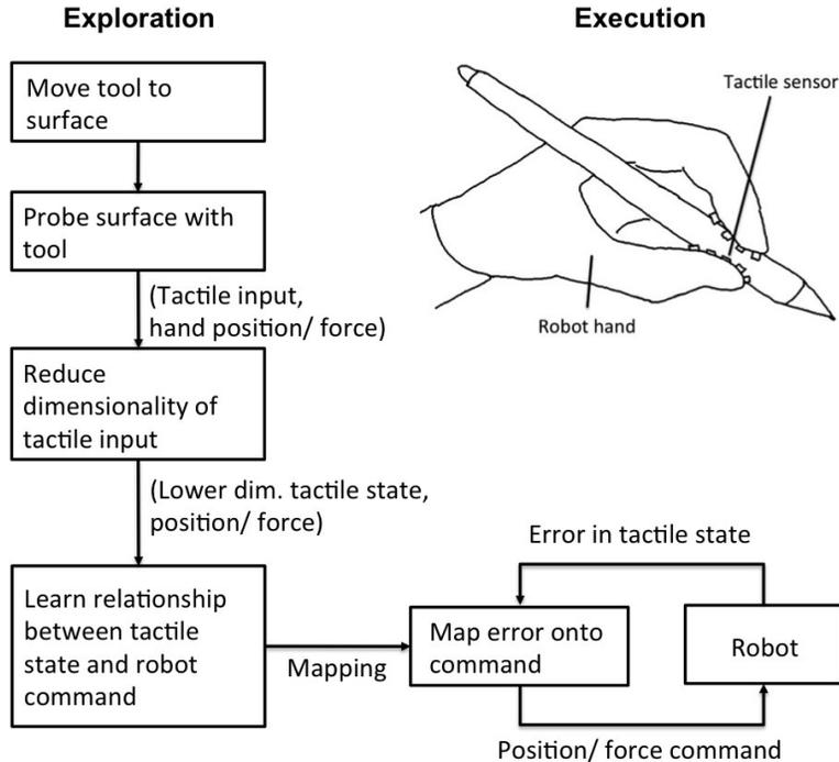
Figure 4: Learning tool-tip control using tactile feedback. This diagram shows the process flow from moving the hand for exploration to learning a sensorimotor relationship. This relationship is then used in closed loop (bottom right) to control the robot hand.
