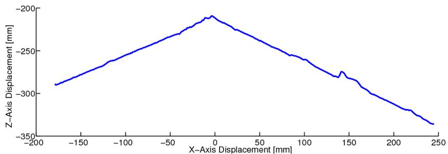
Figure 16: The robot adapted its gripper's vertical position to the slope of the paper surface for drawing. The trajectory was recorded through the robot's internal kinematics (accuracy < 1mm). The trajectory progressed from right to left. The bump in the trajectory reflects a bump in the paper surface (see pictures in Fig. 17).
