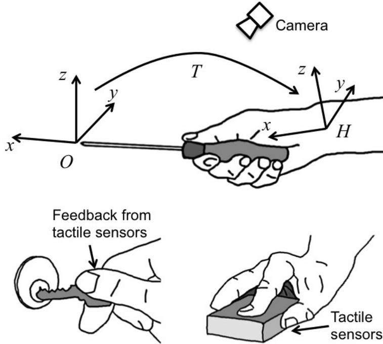
Figure 2: In our framework, we overcome the uncertainty of a grasp by a) obtaining a linear transformation between tool tip frame  $O$  and hand/end-effector frame  $H$  from vision and b) when bringing the tool in contact with a surface, using tactile feedback and learning the mapping between hand control and tactile state.
