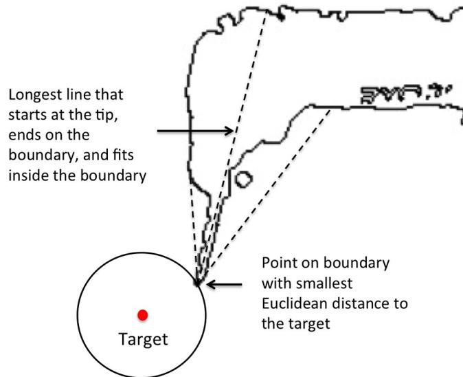
Figure 8: Given the boundary of a tool, we can find the tool tip (closest point on boundary to the target) and its axis (longest line within the boundary, originating at the tool tip).
