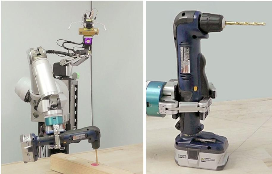
Figure 1: Accurate tool tip control requires adaptation to grasp variability. The red dot on the wooden block is the target for drilling.
