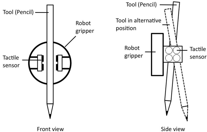
Figure 13: Robot gripper and tool placement. Two 2x2 arrays of tactile sensors were attached to the robot gripper. Here, as tool, we used a pencil, whose position and orientation in the gripper varied between tests (illustrated by dashed pencil contour).
