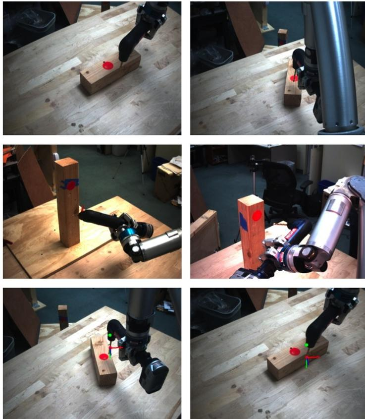
Figure 10: The top four images show examples in which our algorithm failed to detect the tool tip. The bottom left image is an example of a wrong tool tip estimate (red dot). The bottom right image is an example of a wrong estimate of the orientation of the drill bit (blue line, about  $30^\circ$  off). The figure shows the raw images from the Bumblebee2 camera. The lighting varied during these trials.
