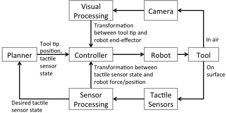
Figure 3: Visual and tactile feedback complement each other in our architecture for bringing a tool to a surface and interacting with the surface.
