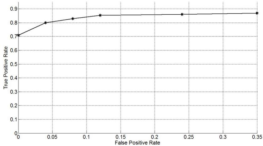
Figure 11: ROC curve for successful tool tip localization. To compute the curve, we varied the threshold for tool tip recognition.
