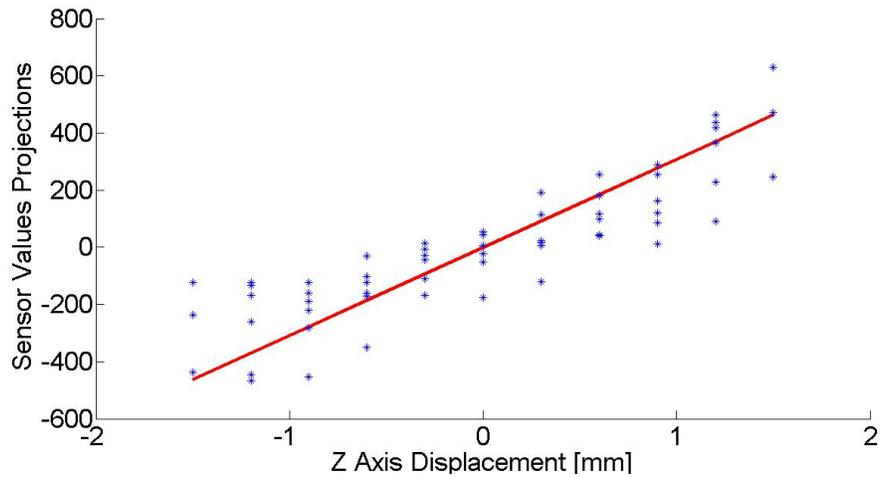
Figure 15: Relationship between hand location (Z-axis displacement) and low-dimensional representation of tactile input (sensor values projected onto first principal component). Recorded values from one exploration trial are shown together with a linear fit to the data (red line).
