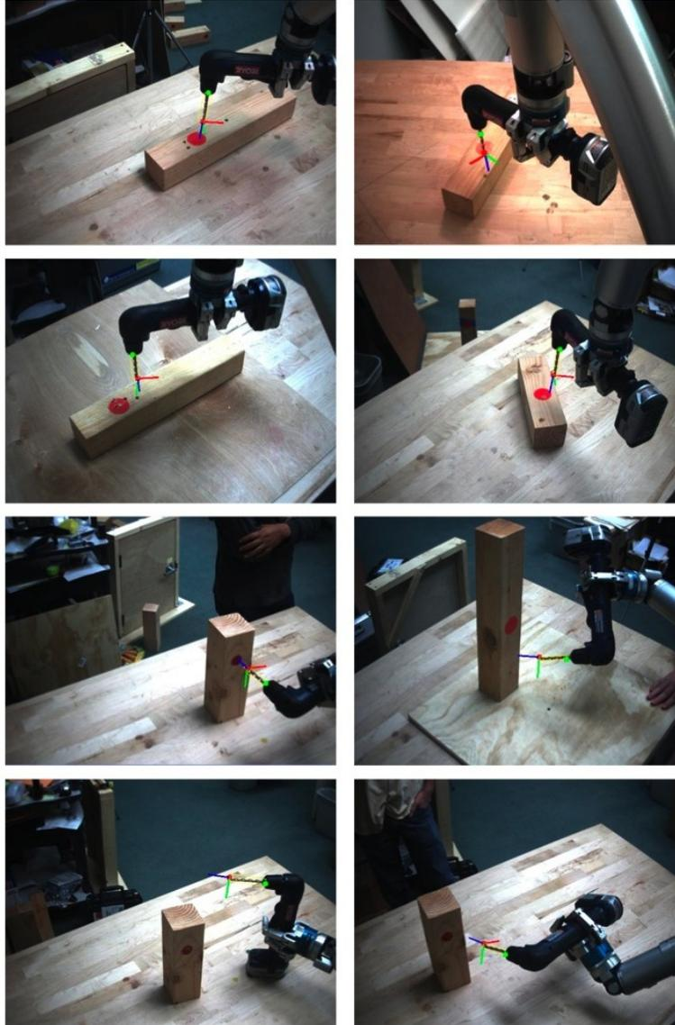
Figure 9: Examples in which our algorithm succeeded to detect and localize the tool tip. The figure shows the raw images from the Bumblebee2 camera. The lighting varied during these trials. The images show overlaid the computed bit tip (red dot) and computed coordinate axes of the drill bit (blue line along the bit axis).
