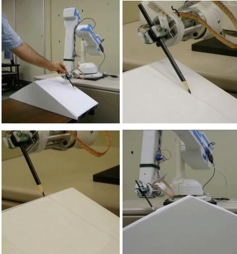
Figure 17: Autonomous drawing with a pencil on a surface of unknown slope. The four images are taken from a video showing the whole drawing sequence. Initially, the pen is placed into the gripper in an arbitrary orientation (the pencil tip has to be able to touch the paper); then, the robot moves the gripper up and down to explore the tactile feedback. Finally, the robot draws on the surface while autonomously adjusting the pencil height.
