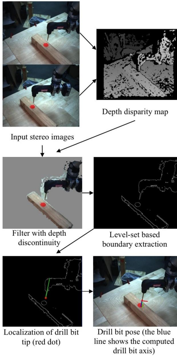
Figure 7: Image processing steps for localizing a tool tip, here, drill bit. The target for drilling is the red dot on the wooden block.
