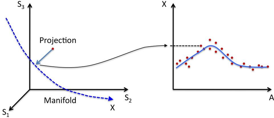
Figure 6: Learning the sensorimotor relationship (illustration - not real data). (Left) Each sensory data point is projected onto the manifold extracted from learning a low-dimensional representation of the sensory input. This manifold is parameterized,  $X$ . (Right) The obtained value from the projection is plotted against the corresponding robot action,  $A$ . Here, another learning method learns the relationship (solid blue curve) between  $A$  and  $X$ .
