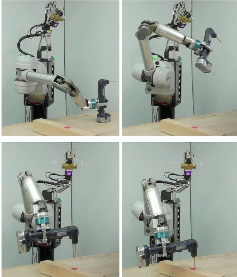
Figure 12: Autonomous drilling. The four images are taken from a video showing the whole manipulation sequence. Initially, the robot autonomously grasped the drill; then, the robot moved the drill towards a target (red dot on wooden block) using visual feedback. Finally, the robot drilled into the wooden block using the augmented Jacobian from joints to drill bit position.
