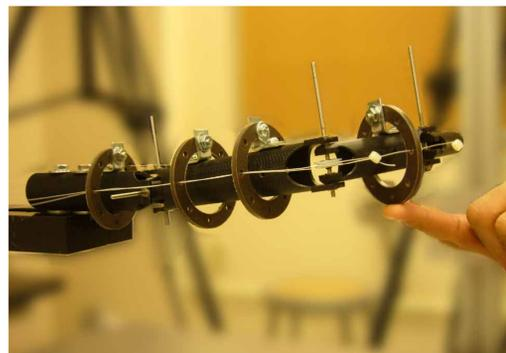
The four-degrees-of-freedom mechanical finger is equipped with polyoxymethylene disks that allow alternative tendon-routing paths. We mimicked the main routing paths in the index finger.
