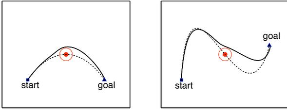
**Fig. 1:** Movement generation with potential field (solid curve). The original movement is shown with a dashed line.
