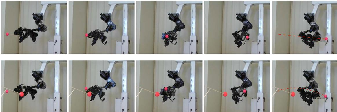
**Fig. 3:** Obstacle avoidance with Sarcos Master Arm. The first row shows the reproduction of a demonstrated movement, and the second row shows the result of obstacle avoidance with the potential field.
