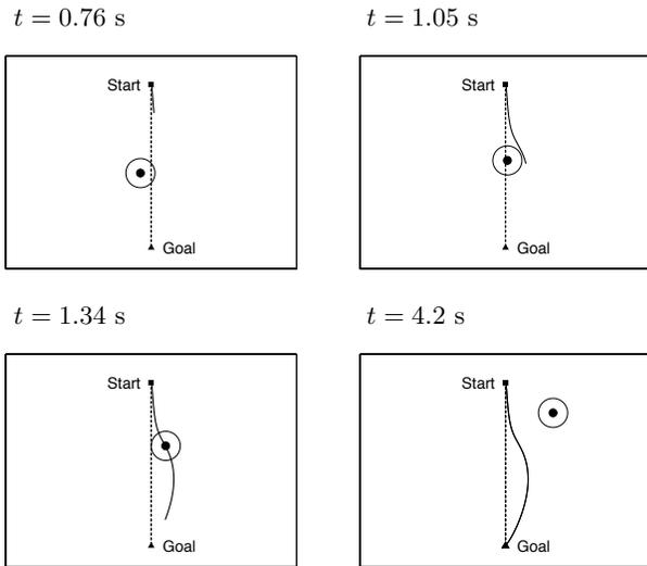
**Fig. 2:** Movement generation with potential field and moving obstacle. Different time steps of the movement are shown. The obstacle moves from bottom left to top right of the workspace.
