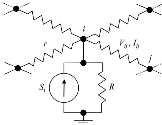
Figure 1: A circuit model. Each node  $i$  is connected to a current source  $S_i$  and a load resistor  $R$ . The grid lines have a resistance of  $r$ .
