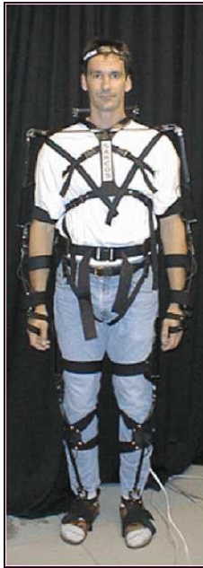
Fig. 1 Thirty-degrees-of-freedom sensuit used to capture human kinematic movement data
