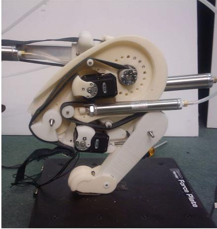
Fig. 6. Realization of the Cheetah Robotic Limb
