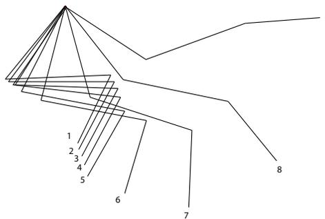
Fig. 9. Digitized video recording of movement of leg during the dynamic kick test. The stick figures above represent 9 video frames 33 ms apart. All data is with respect to the hip. At frame 7, the leg is still on the ground. At frame 8 the leg is airborne.
