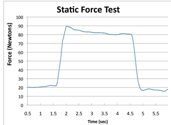
Fig. 7. Static force test. The robot is held down by an experimenter and 130 psi is applied. The weight of the robot is about 22 Newtons.
