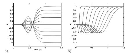
Figure 4: Illustration of invariance properties in the discrete dynamical systems, using the example from Figure 1. (a) The goal position is varied from -1 to 1 in 10 steps. (b) The time constant  $\tau$  is changed to generate trajectories from about 0.15 seconds to 1.7 seconds duration.
