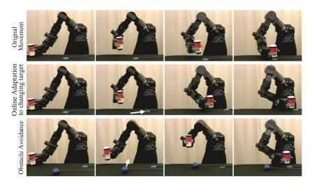
Figure 9: Sarcos slave robot placing a red cup on a green coaster. The first row shows the placing movement on a fixed goal with a discrete dynamical system. The second row shows the ability to adapt to changing goals (white arrow) after movement onset. The third row shows the resulting movement as a blue ball-like obstacle interferes with the placing movement, using the coupling term from equation 3.2.
